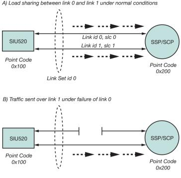
Figure 3. SIU Connected to Adjacent Node with Two Links in Link Set
